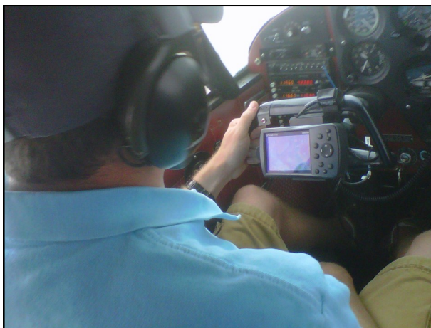
Harrison Hoffman flying the Piper Comanche for the PGCD Precipitation Enhancement Program. The GPS helps Hoffman to navigate his track within the District, and also shows real time radar data which helps in communicating with the meteorologist.
