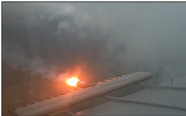
Hygroscopic flare, made by Ice Crystal Engineering, burning during a mission in the South Texas Weather Modification Association target area. This hygroscopic flare was composed of 1,000 grams of CaCl.
